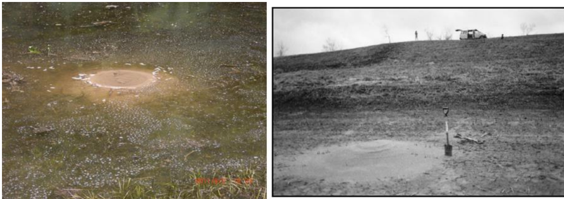
Figure 2. 8 Sand boil during flood event in Mississippi River Valley (Li et al. 1996; Alfortish et al. 2012).
