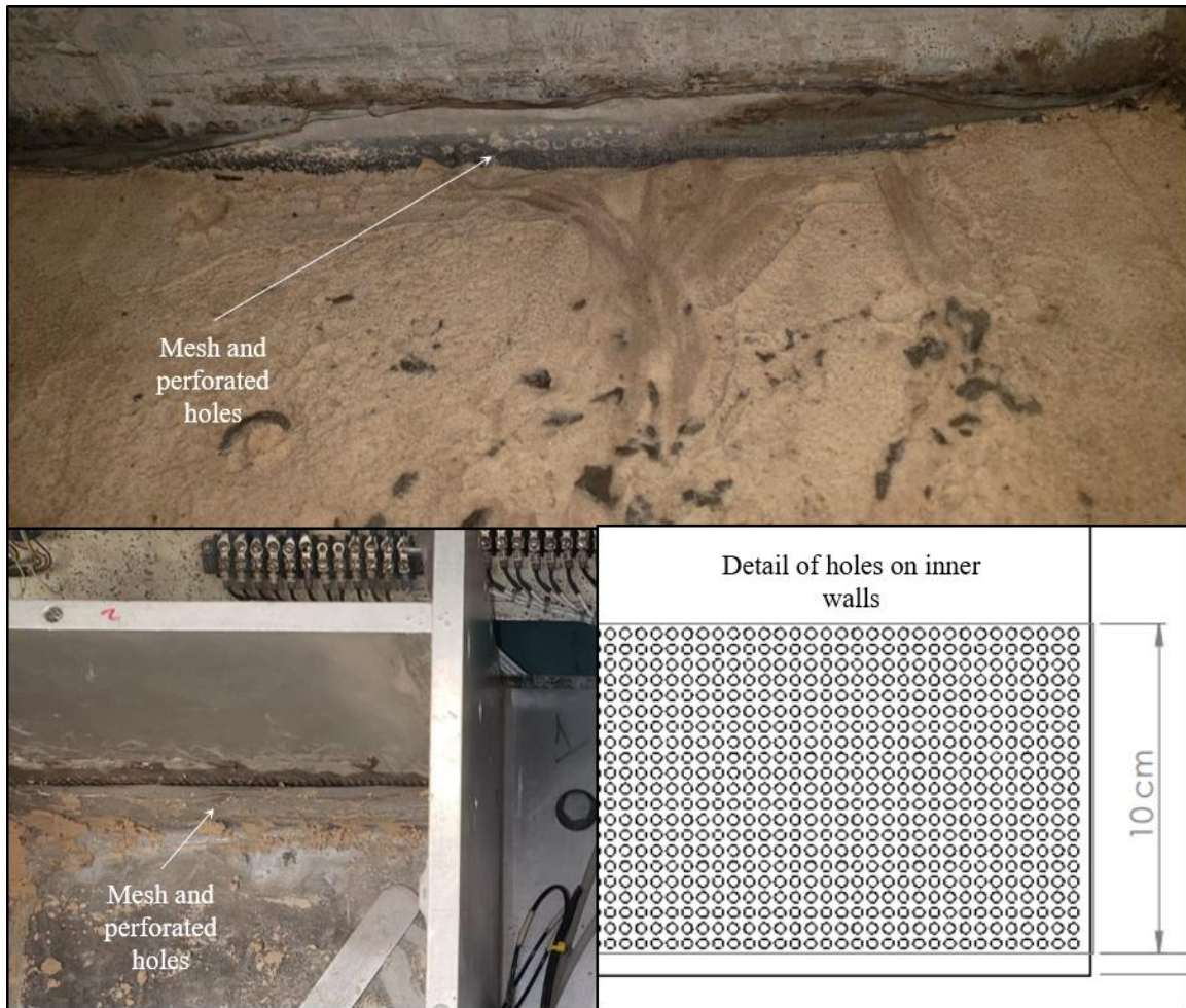
Figure E. 1 Stainless-steel mesh and lateral perforated holes.
