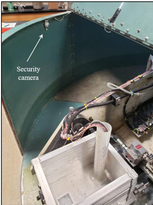
Figure A. 15 Fixed camera to monitor the arm assembly.
