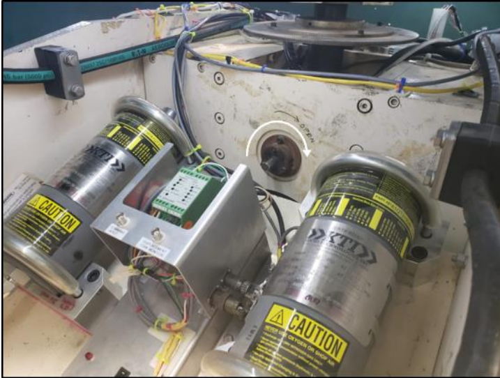
Figure A. 23 Centrifuge balance lock rod.
